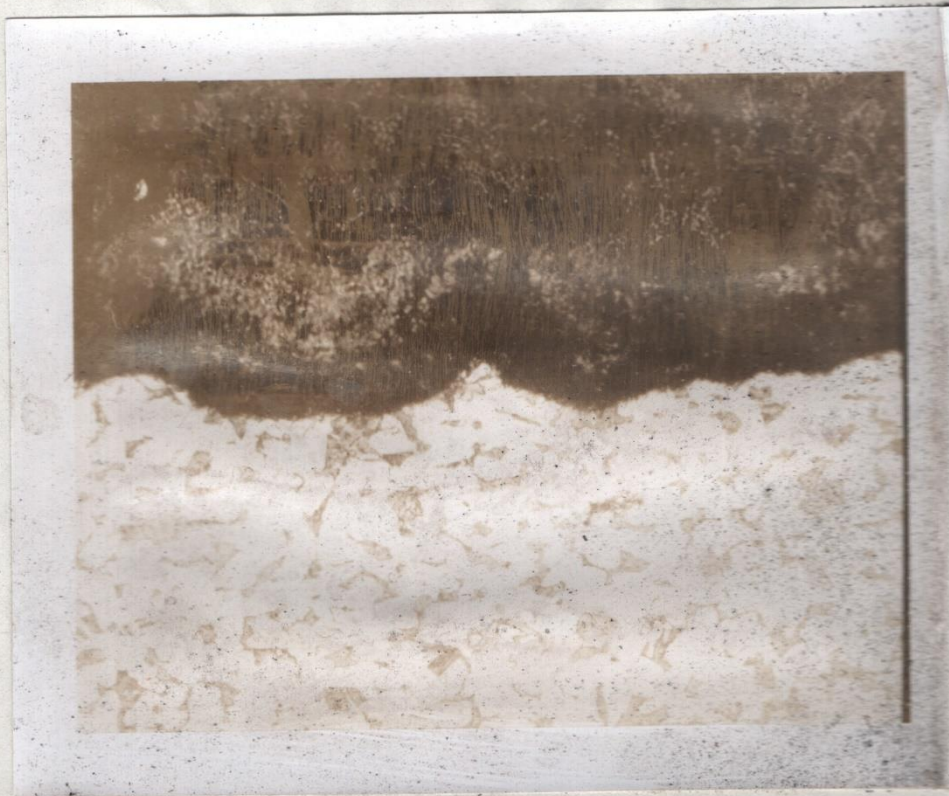
Figure 1. Uniform Corrosion on COG Line ( \times 200 )
